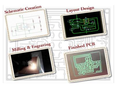
This was followed by Gerber and G-Code generation using Nvis Software which is required by the Nvis PCB Prototype Machine. The students were taught to generate Gerber and G-Codes for Milling, Engraving and Drilling, which were then imported to the PCB Prototype Machine. The students were shown how to use the Nvis PCB Prototype Machine for the PCB creation. The coordinators for the workshop were Prof. Flavia Leitao and Prof. Melba D'Souza.
